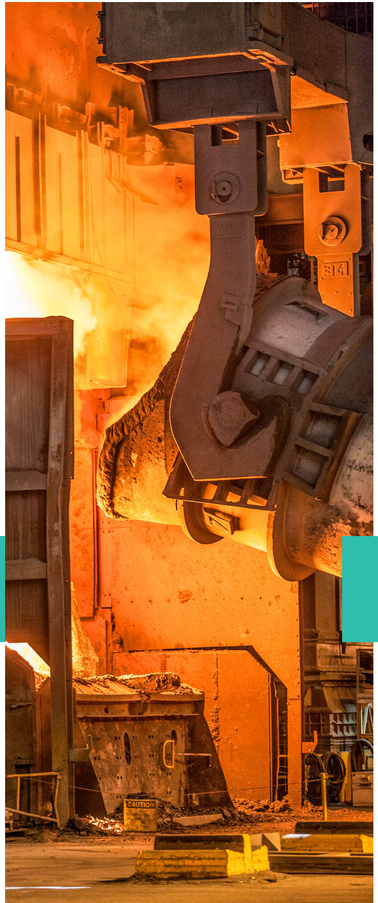
Image: Basic Oxygen Steelmaking Facility at Port Kembla Steelworks Australia. A crucial piece of BlueScope's manufacturing infrastructure in Australia which converts liquid iron and scrap into steel. | Source: BlueScope Steel
